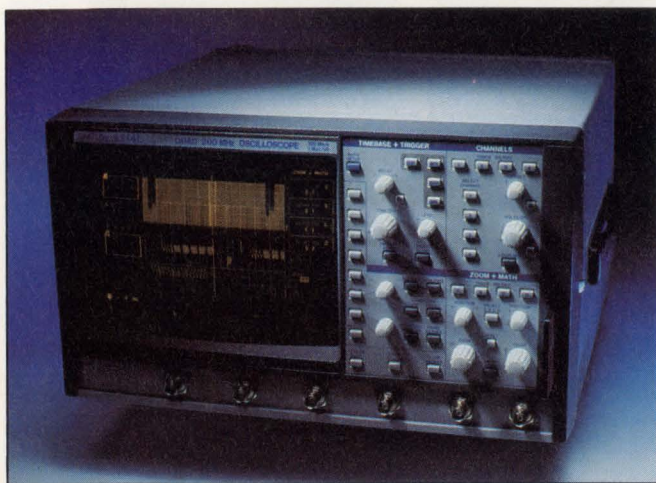
A 1-Msample memory doesn't make LeCroy's 9300 scopes large or odd in appearance. Casual observers may even miss the small slot at the lower right that accepts credit-card-size memory cards that store waveforms and setups.
