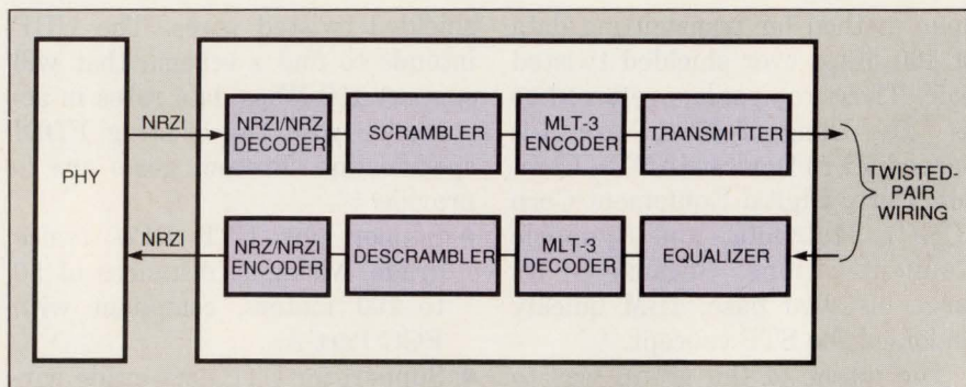
Fig 2—This functional block diagram illustrates a typical method for implementing the FDDI Physical Medium Dependent (PMD) protocol using scrambled MLT-3 coding over copper wire.
