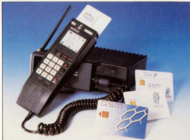
Applications of smart cards in Europe include controlling access to cellular-phone services. Smart cards provide security and other benefits that magnetic-stripe cards do not. (Photo courtesy Gemplus Card International)
