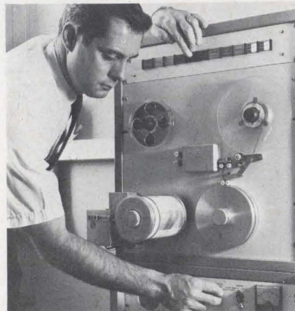
High-speed spectrograph, developed at Bell Telephone Laboratories, works directly from standard magnetic tape.
