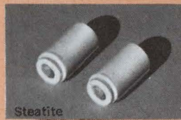
Steatite Length .500 \pm .003 Shank O.D. .235^{+.000}_{-.005} Hole .139^{+.006}_{-.000}
