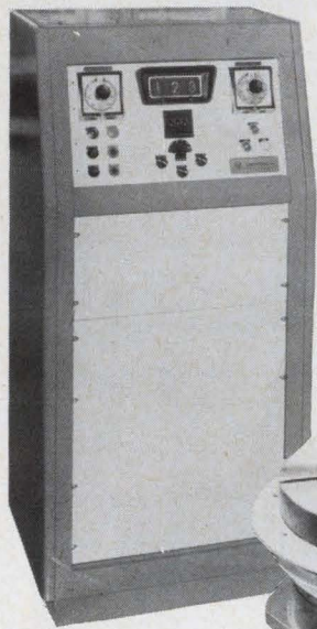
24" ULTRADEX with visual read-out remote control console for automatic indexing.
