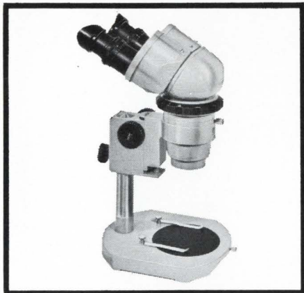
Stereo Zoom Microscope SMZ 4X to 120X
