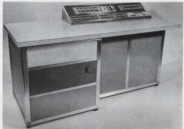
3. Gate reduction possible through the use of threshold logic was demonstrated in the design of this small, general-purpose computer built in 1964 at General Electric Research Laboratories. The results are summarized in the Table in terms of the gate requirements.
