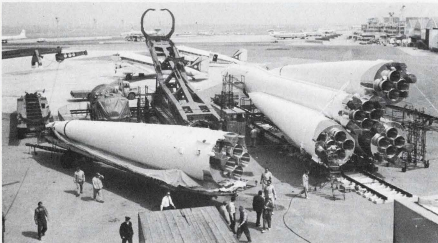
Soviet space vehicle boosters , of the type that lifted the manned Vostok and Cosmos satellites into orbit, are displayed at a British air show.
