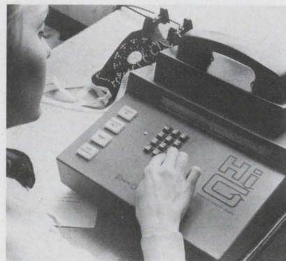
Simple pushbutton telephone-type keyboard eases interface for input and output information.
