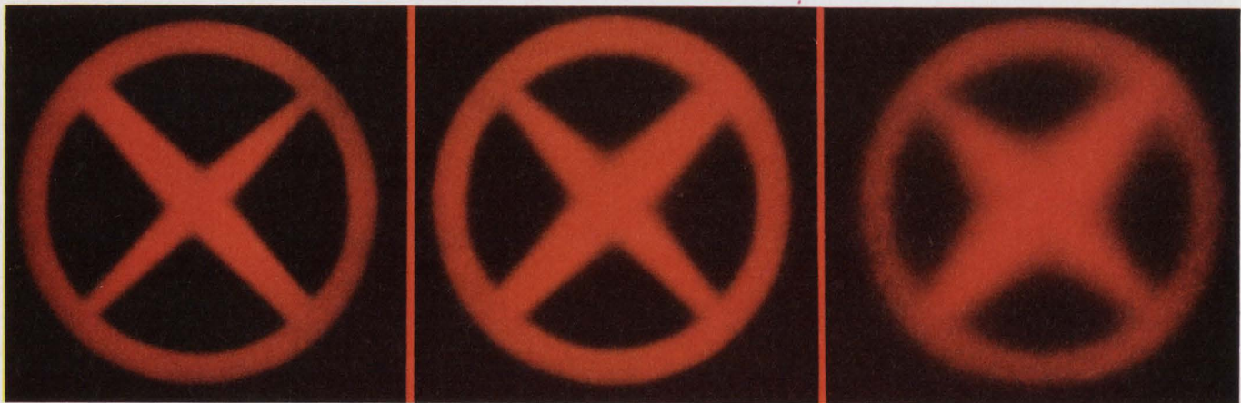
Reducing the redundant information content of a hologram also decreases either the field of view or the resolution (as shown here in successive data reduction
