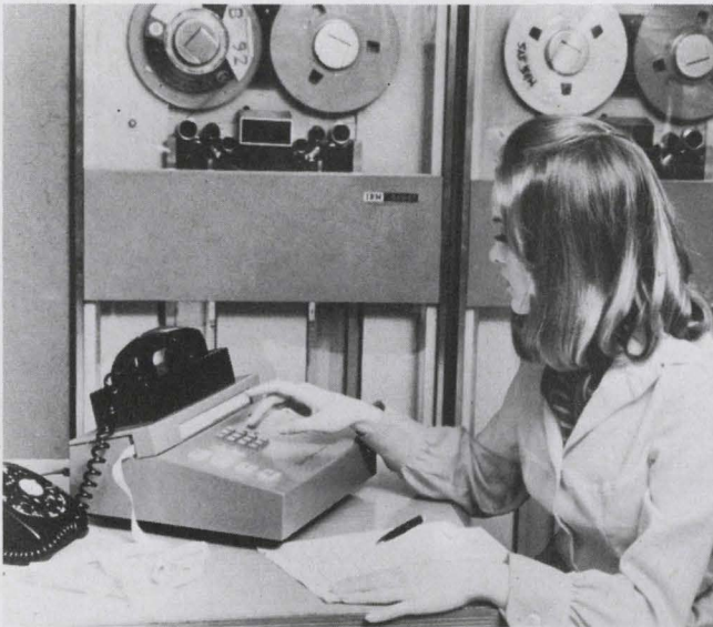
Hard-copy computer terminal handles data at rates to 10 characters per second, p. 114.
