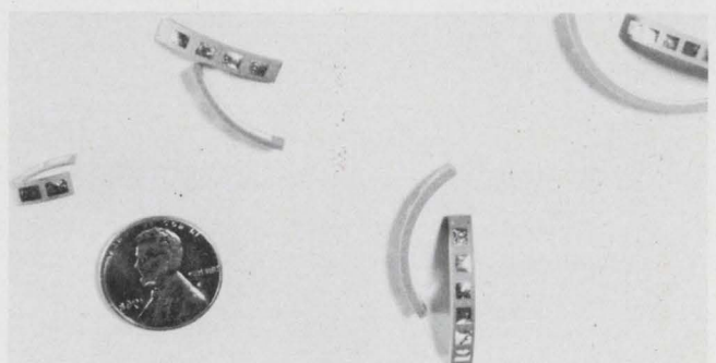
Curved-bank ceramic capacitors are highly complex in their construction. Both single-layer and multilayer devices can be intricately formed.
