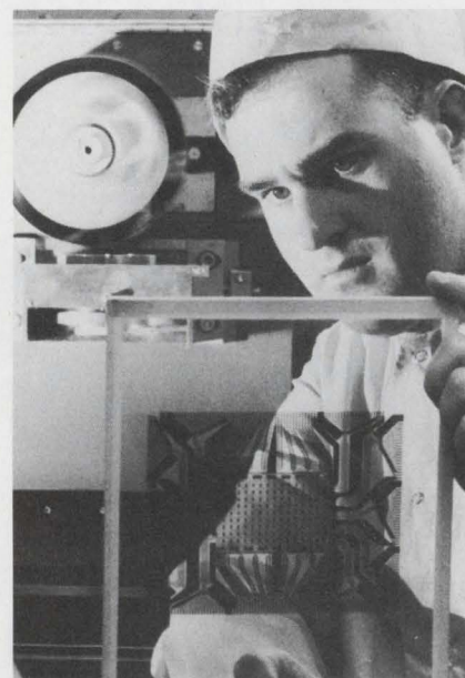
Laser beam and 10-sided rotating mirror cut time to one-sixtieth for drawing mask patterns for ICs.
