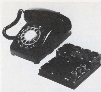
High density packaging compresses memory, CPU and I/O units into this rugged subminiature computer.
