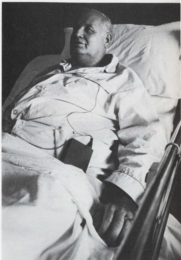
2. This biomedical transmitter, in use in Overlook Hospital, Summit, N. J., is larger than ideal size. Additional design is necessary to make it small enough for young children or for transmission of several channels of medical data.
