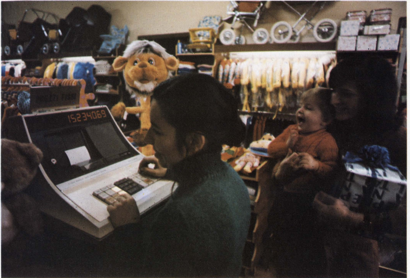
Point-of-sale systems are beginning to replace electro-mechanical cash registers in retail stores and super-
