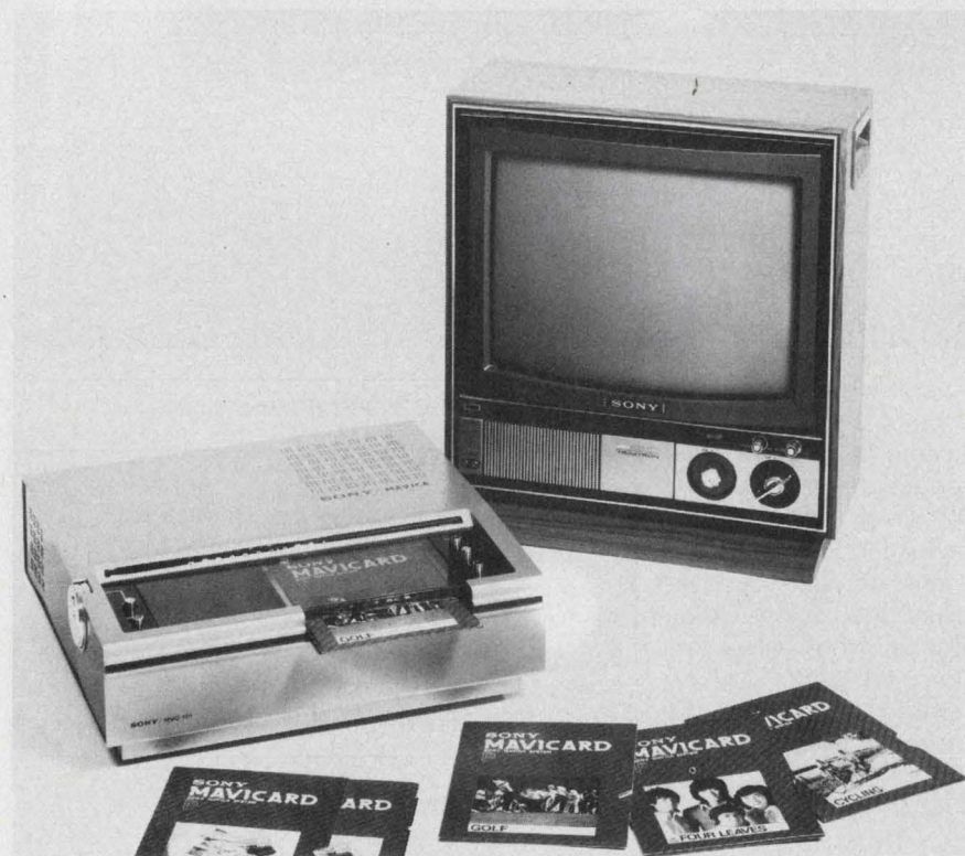
Sony Corp.'s Mavica video playback unit uses a 176-by-226 mm magnetic card that can store 10 minutes worth of video and stereophonic information.
