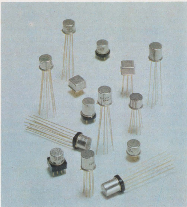
These miniature TO-5 and square header relays from Teledyne Relays can handle currents up to about 1 A and provide up to two form C sets of contacts.
