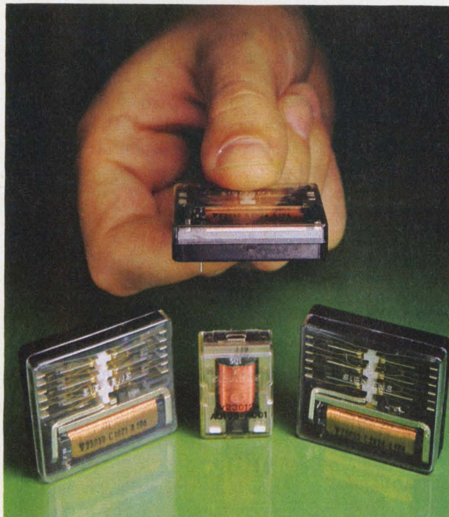
Low-profile relays made by Siemens are designed for mounting on printed-circuit boards and have a height above the board of only 0.5 in.
