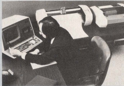
Trio of new products from Wang Laboratories consists of (from left to right): 2200 PCS minicomputer, \mu P-based "virtual drum" plotter and 120-cps serial matrix printer.
