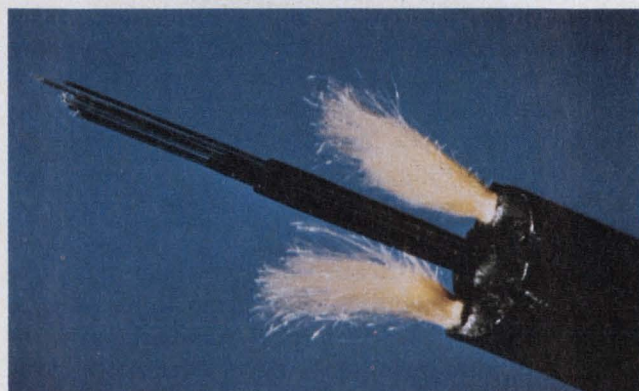
A six-fiber optical cable, Corning's Corguide, was developed for military field use. The tiny central fibers are protected by a tough, extruded jacket, shown in cross-section. Each fiber has a max 20 dB/km loss.
