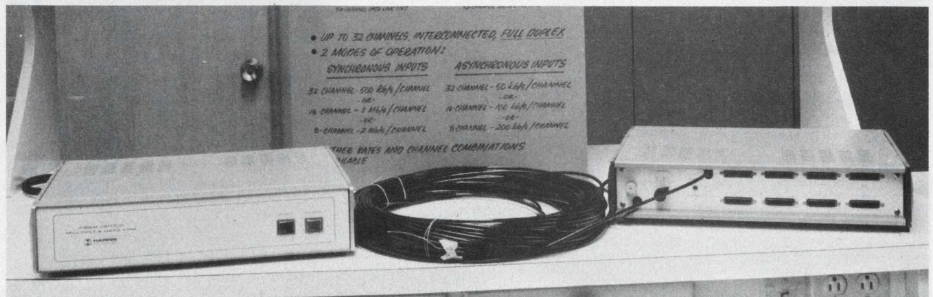
This 32-channel digital data link , by Harris, is suitable for computer-to-peripheral installations up to 1500 feet apart. The system uses Corguide and operates at 16
