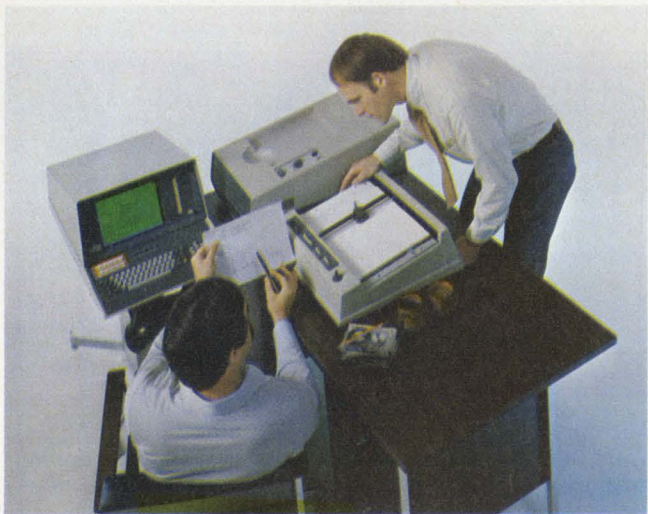
Interactive digital plotting is a new concept brought to realization by the microprocessor. The Tektronix 4662 digitizes and transmits its pen position.
