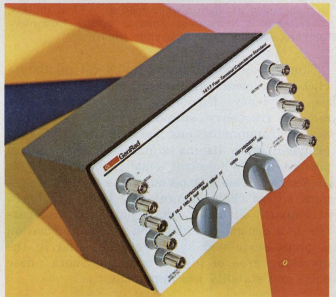
Seven ranges of capacitance from 1 \mu F to 1 F can be selected with the GR 1417. The four-terminal standard also acts as a standard for dissipation factor.
