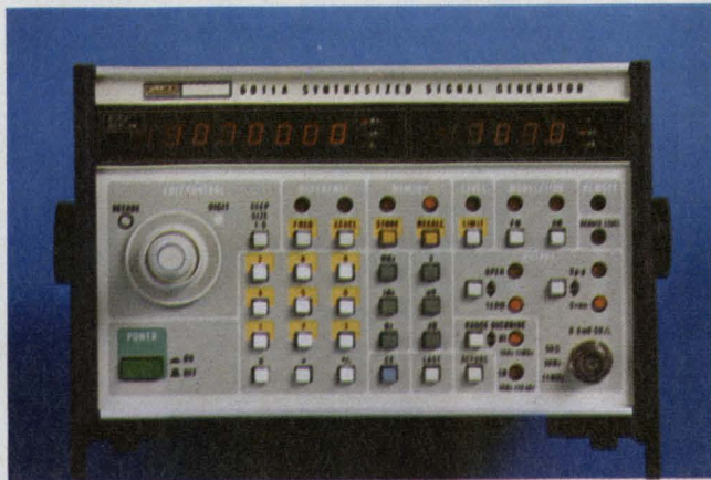
The new look in signal generators: Fluke's 6011A stores frequencies and amplitudes and lets the user edit or modify the output from a keyboard.
