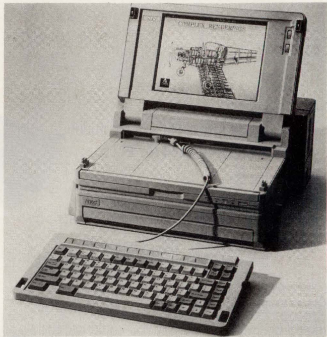
3. CONNECTING TO A STATIONARY docking station is NEC's Prospeed SX/20, a 386SX-based laptop computer. With the docking station, users can add expansion cards, drives, or other peripherals through the interface slots.
