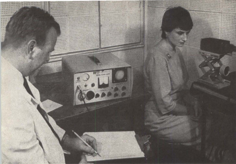
Flicker-fusion tester in use. Ammeter indicates light brightness, cathode-ray tube presents ratio of on and off times
