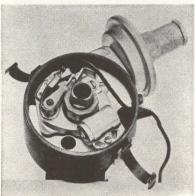
Distributor cam is replaced by toothed wheel that generates pulses in magnetic pickoff
