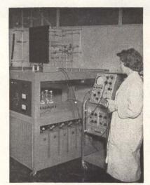
System for rapidly adjusting film resistors could be used to adjust resistances in microcircuit films and in composite printed circuits
