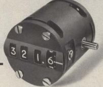
Direct visual counter display with large numerals enables lower valued increments of angles to be easily read in terms of minutes and seconds of arc. Precision design, rugged construction, durable materials. With odometer or Geneva drives. Temperature range -65°C to +90°C; meet military requirements for shock, vibration, case size.
