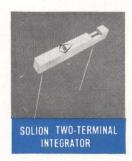
SV series, .002 to 5  $\mu a$ input, output 0-60 mv calibrated proportional to time integral of input. Ultra miniature, ex-
