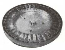
Bottom view of wave antenna switching unit
