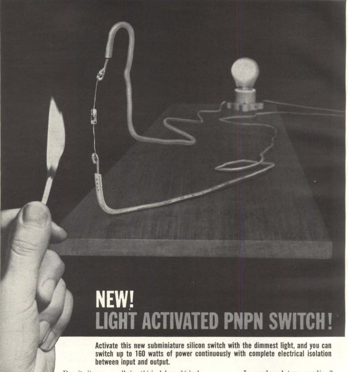
Despite its very small size ( $\frac{1}{3}$  inch long,  $\frac{1}{8}$  inch diameter) the new ZJ235 is rated at 400 ma d. c. in latching applications, with a surge current rating of 5 amps. Voltage ratings are from 50 to 400 volts. A short impulse of light of as little as 80 foot candles will trigger the ZJ235 into conduction.
