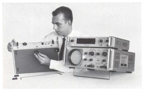
Feet furnished with modular instruments snap quickly in place without tools, permit "no-slip" stacking. You have a "rack-less rack" that places a maximum of easily arranged instrumentation immediately at hand. Shown: Models 457A AC/DC Converter, 120B Oscilloscope, 5532A Counter.
