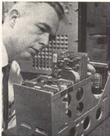
Computer's transistor circuits are contained on six plug-in cards
