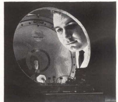
PHYSICIST checks alignment as x-ray gun is fitted to specimen-chamber porthole
