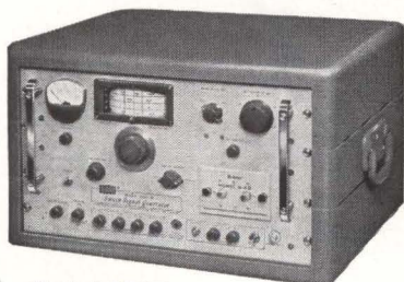
Model 900B Super Sweep Generator
