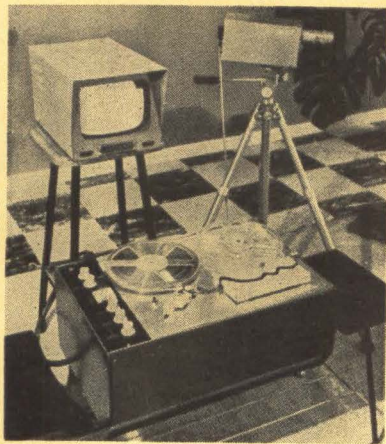
TELCAN equipment (Aug. 16, p 7) records tv programs on standard \frac{1}{2} -inch tape. Manufacturer sees replacement of home movies with "canned" home television.
