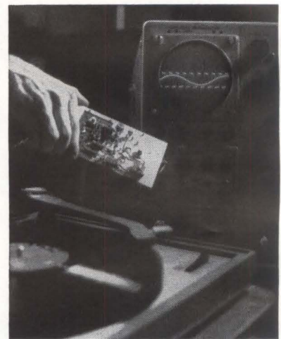
SCOPE SHOWS sine-wave input and rectangular output simultaneously, for display purposes. The pocket-sized hi-fi amplifier is connected to the scope, but record pickup in foreground is not
