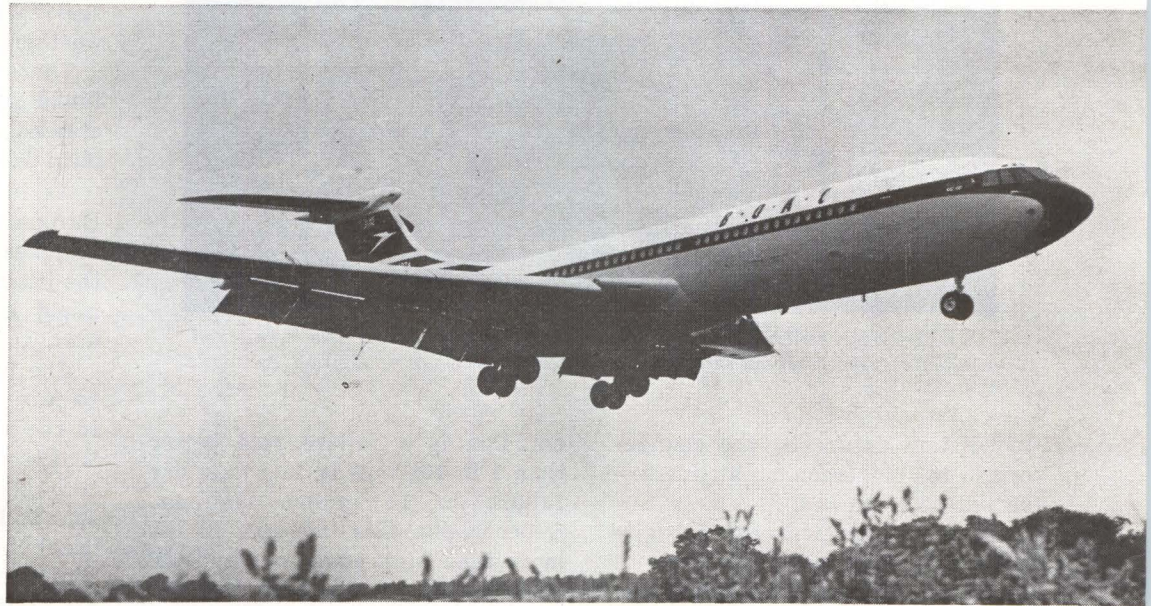
VC 10 LINER comes in for a landing during trial run of British Autoland System
