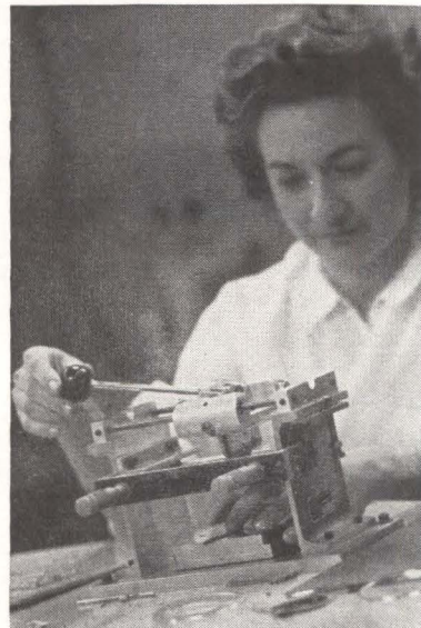
AUTOMATIC processing equipment is employed in the Helipot Ceramic Engineering department to form the basis of cermet resistance elements
