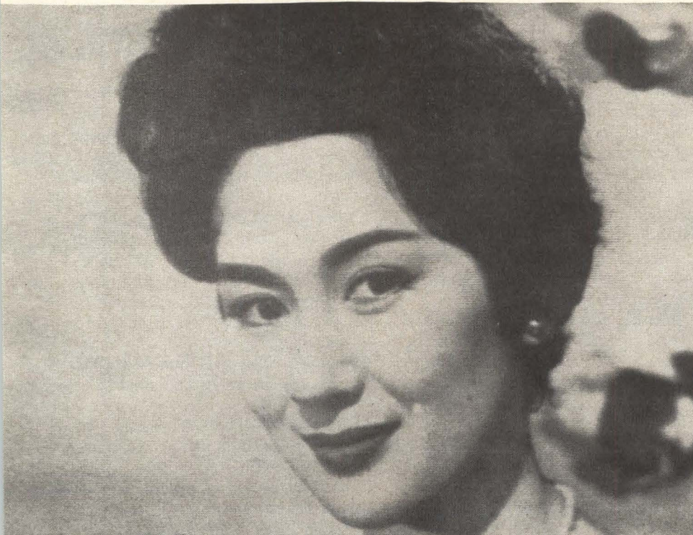
REPRODUCED IMAGE from pickup storage tube, with 1,500-lux illumination, f/2 lens opening, 0.1-sec exposure—Fig. 4
