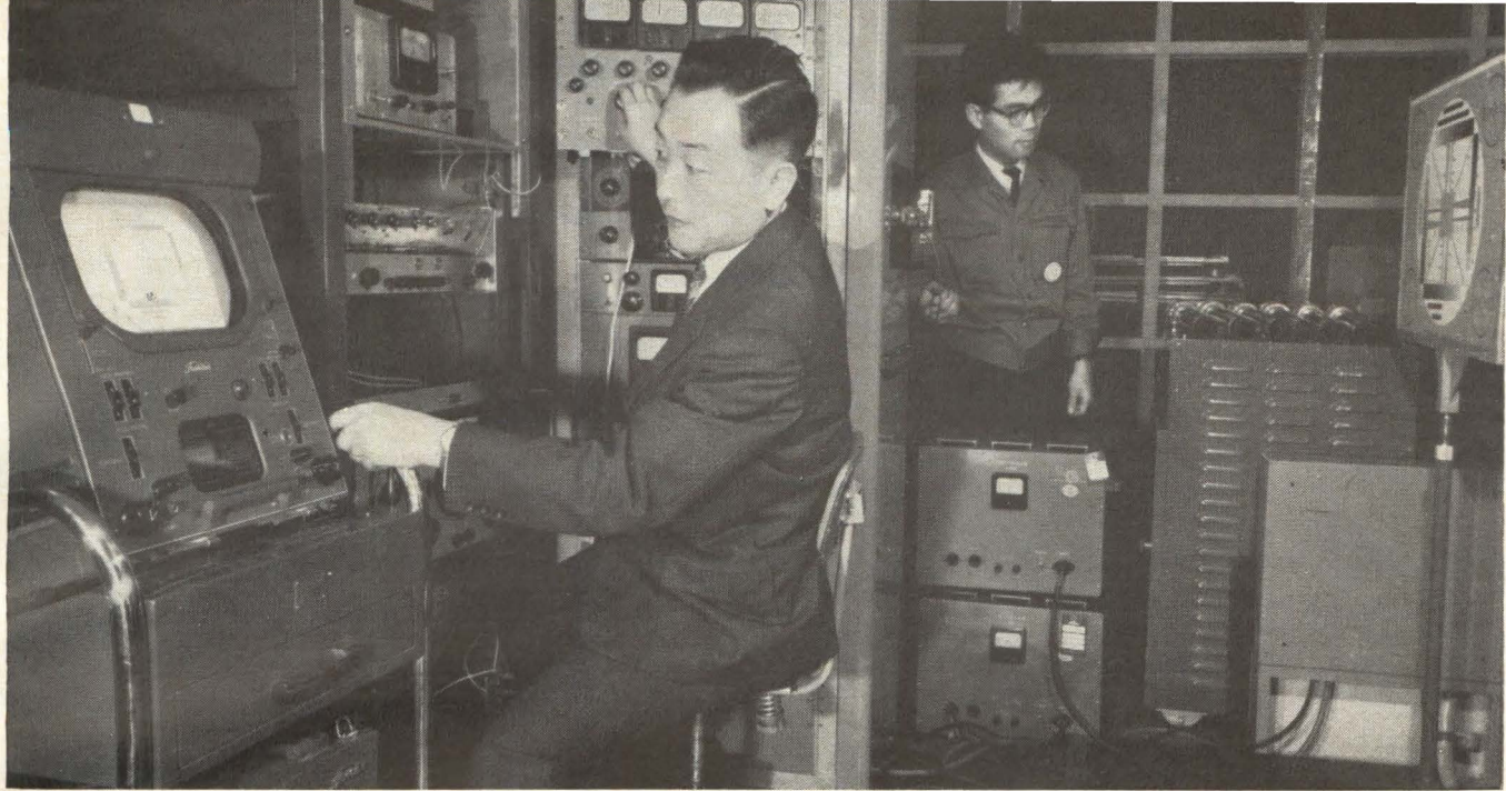
AUTHOR Odagawa observes monitor display of test pattern image from pickup storage tube signal
