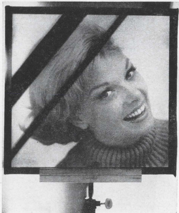
Flat panel display developed by the Librascope group of General Precision, Inc., a subsidiary of General Precision Equipment Corp., has variable persistence and erasure capability. Black streaks demonstrate selective erasure by an infrared light source.
