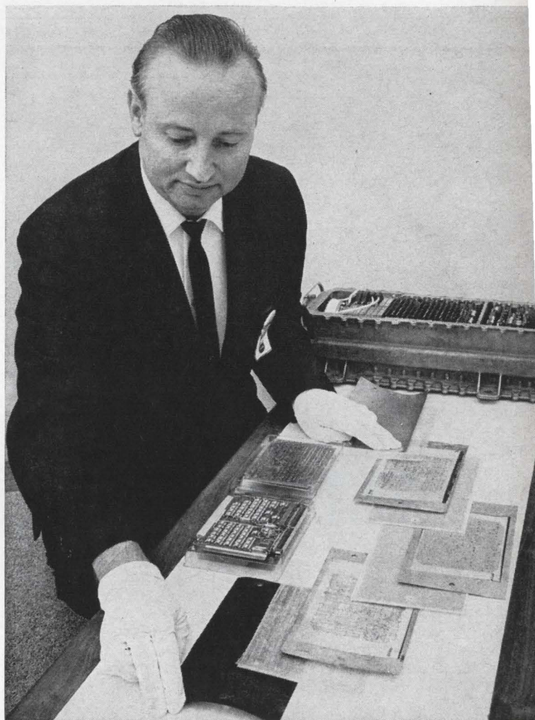
Individual layers of a multilayer board are spread out on a table. Two boards are directly in front of the author; a D37 computer for the Minuteman 2 missile system is at his left.
