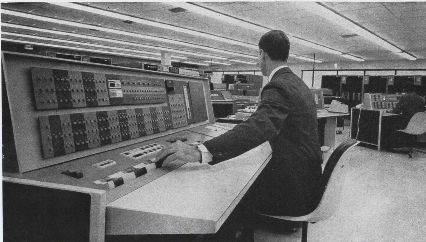
Time sharing is exemplified by this airline reservation system, American Airlines' Sabre installation in Briarcliff Manor, 30 miles north of New York City. The computer is an IBM 7090; it can reserve a seat on any American Airlines flight almost a year in advance, in less than three seconds—and handle 2,100 such requests every minute.
