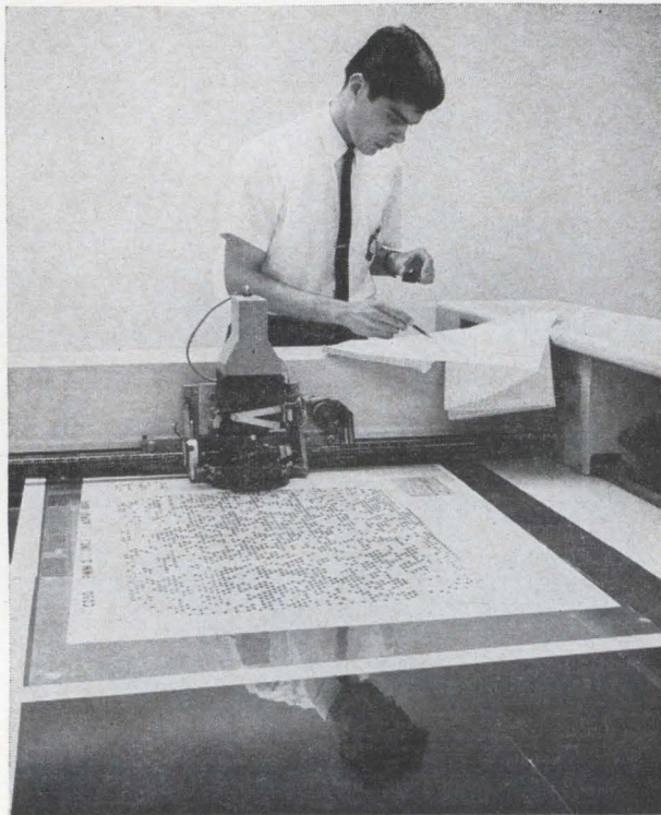
Master negative for a board layer is prepared automatically with this computer-programmed drafting machine. Standard parts of the pattern, such as pads and line segments, are generated photographically.
