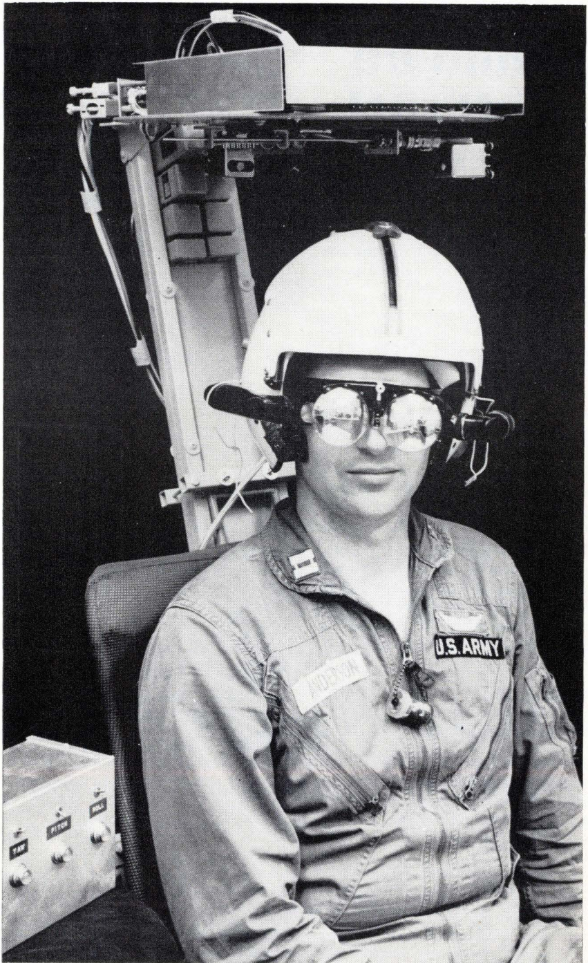
Pilot views on his special lenses what his low light-level tv camera picks up in the dark. He can also look through this display at the normal night scene.
