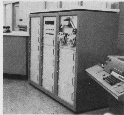
Prober. Machine is designed to test as many as 3000 terminals at a time.
