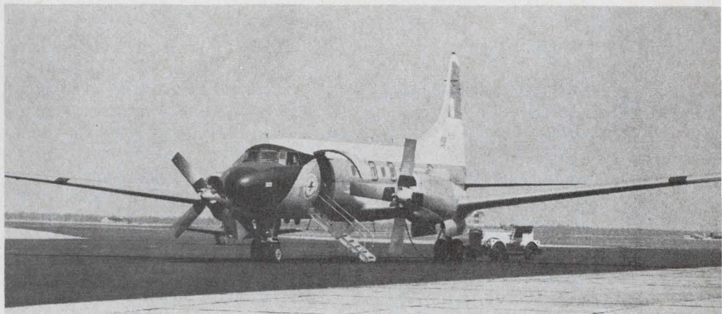
New home. Turboprop Convairs, outfitted with the Seal system, will eventually replace the FAA's fleet of DC-3's in making low-altitude checks of ground-based navigation aids like VOR, Tacan, and Vortac.
