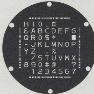
Fig. 3. Stencil character screen from 2" monoscope can be custom-designed to your requirements.
