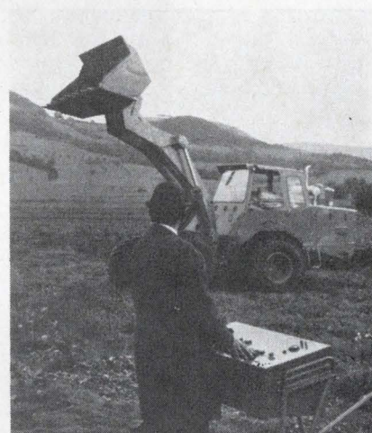
On its own. Scoop loader's 28 different functions are controlled from remote transmitter.
