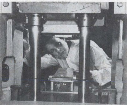
Aligned. Finally, the die is put in a punch press to stamp a circuit on a substrate from a sheet of foil.
