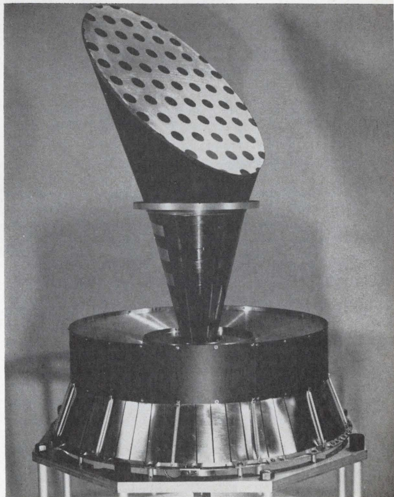
Around the horn. Mechanically despun antenna has an elliptical reflector plate supported by a fiberglass shell resting on a conical horn. The motor is out of sight beneath the protective support structure.
