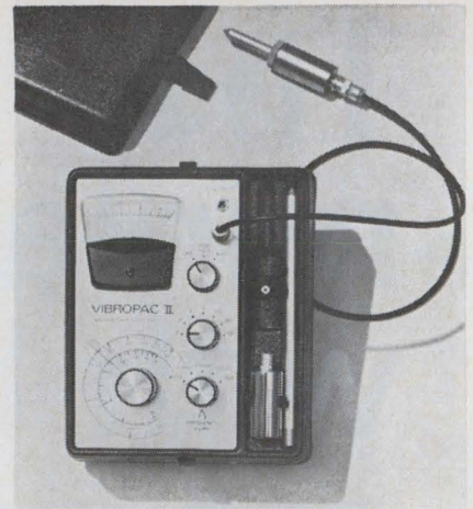
Feeling the rumbles. The tip of the probe is held against the machine.
