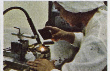
TIG (Tungsten inert gas) welding process is used to seal headers to cases.
