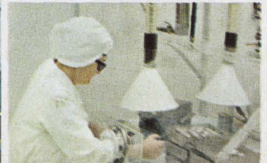
Sealing in controlled atmosphere follows evacuation in vacuum ovens.
