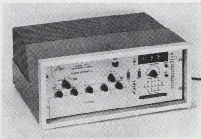
Programmable. Comparator circuits check IC against program board.
