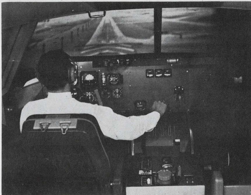
In depth. Flight simulator is used by Lockheed pilots to check out full-scale flight-station mockups of avionics systems proposed for L-1011 airbus. Terrain image is furnished by a closed-circuit television.
