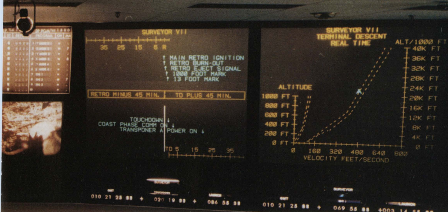
Surveyor support. Display system at Jet Propulsion Laboratory can monitor four space missions simultaneously. In January, the system backed up the Surveyor 7 mission by providing real-time displays.
