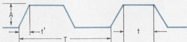
Trapezoidal pulse. A steep rise time, t' , creates high harmonics with large amplitudes.
