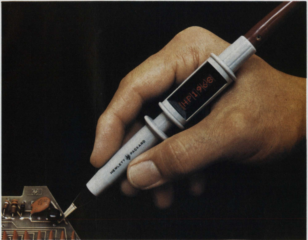
Handy. Small size of solid state unit can be a convenience, as in this experimental probe display, which puts measurement data at the operator's fingertips.
