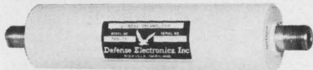
TPA-70 and TPA-73 S and L-Band Preamp amplifiers. S-band: 6 db. Maximum noise: 20 db. Minimum Gain/ L-Band: 5 db. Maximum Noise: 20 db. Minimum Gain/ No Parametric Oscillation with Signal Overloads/ High immunity to strong signal burnouts/ Power output for 1 db Amplitude Compression: -5 db minimum.
