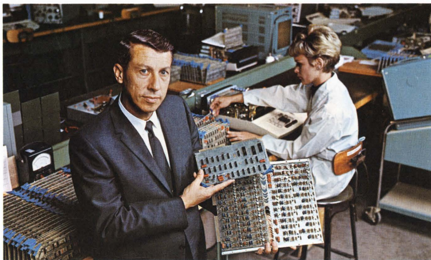
Smaller circuit boards, made possible by MSI and multiple-gate ICs, enabled Friden engineers to develop high-performance low-cost calculators, with both electronics and printer in a single chassis. Here, R. A. Ragen, Friden's Director of Engineering compares a new MSI/IC circuit board with one of the larger functional equivalents required in an earlier all-discrete-component model. In the pre-assembly checkout area (background), an 1151 Calculator performs final screening of hundreds of circuit boards each day.
