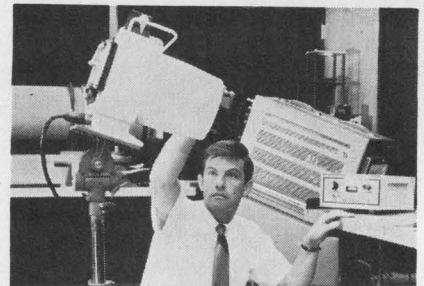
Broad outlook. The T-6 scans a 10° by 10° field covering 10,000 points.
