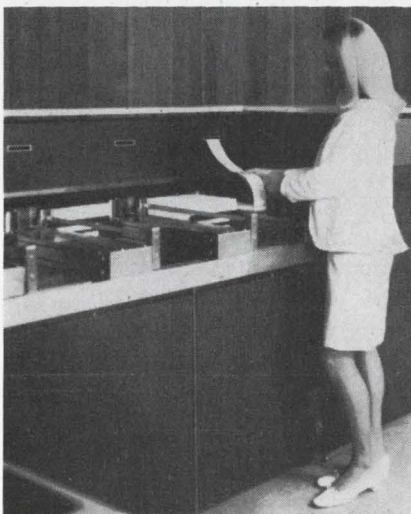
Fibers for reading. Documents travel from the vibrating table, past the de-doubler to the scanner, and on to the sorter (above). In the scanner, images are projected onto a column of 80 optical fibers.
