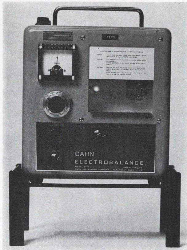
Ultra-microbalance. This instrument weighs single cores to an accuracy of half a microgram.
