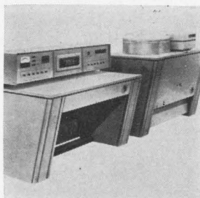
Automatic r-f batch sputtering system is for IC and semiconductor manufacturers. It can process up to 4,000 square inches of substrate material in one pump-down. Typical sputtering rates for electronic applications vary from 100 to 400 angstroms per minute for nonmetallic materials and 300 to 700 angstroms for metals and alloys. Materials Research Corp., Orangeburg, N.Y. [427]
