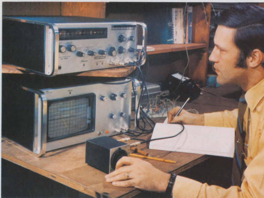
Trial sweep. The frequency generator, top, is sweep-testing a tunable bandpass filter, and output is shown on the oscilloscope.
