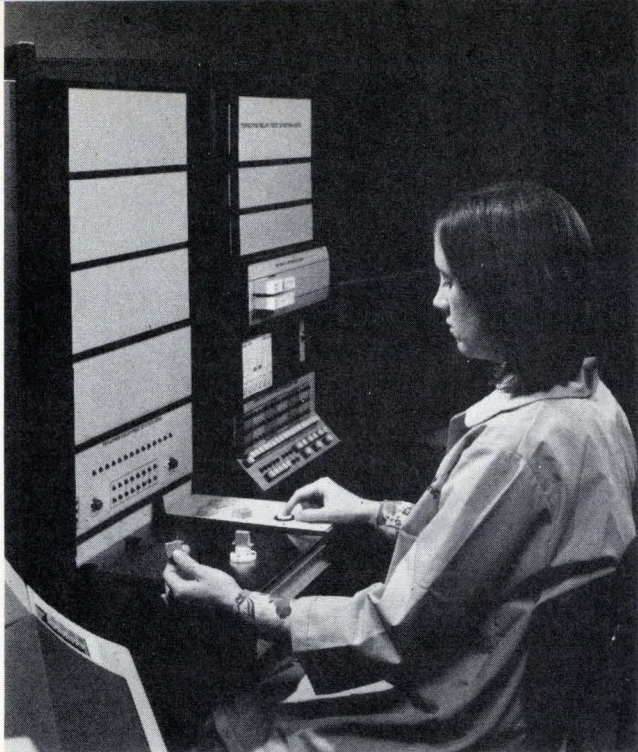
5. Component tester. Teradyne's K167B relay-test system is designed to examine a relay in any sequence with a single insertion. The system provides various types of hard-copy data that is valuable to the relay user and manufacturer.
