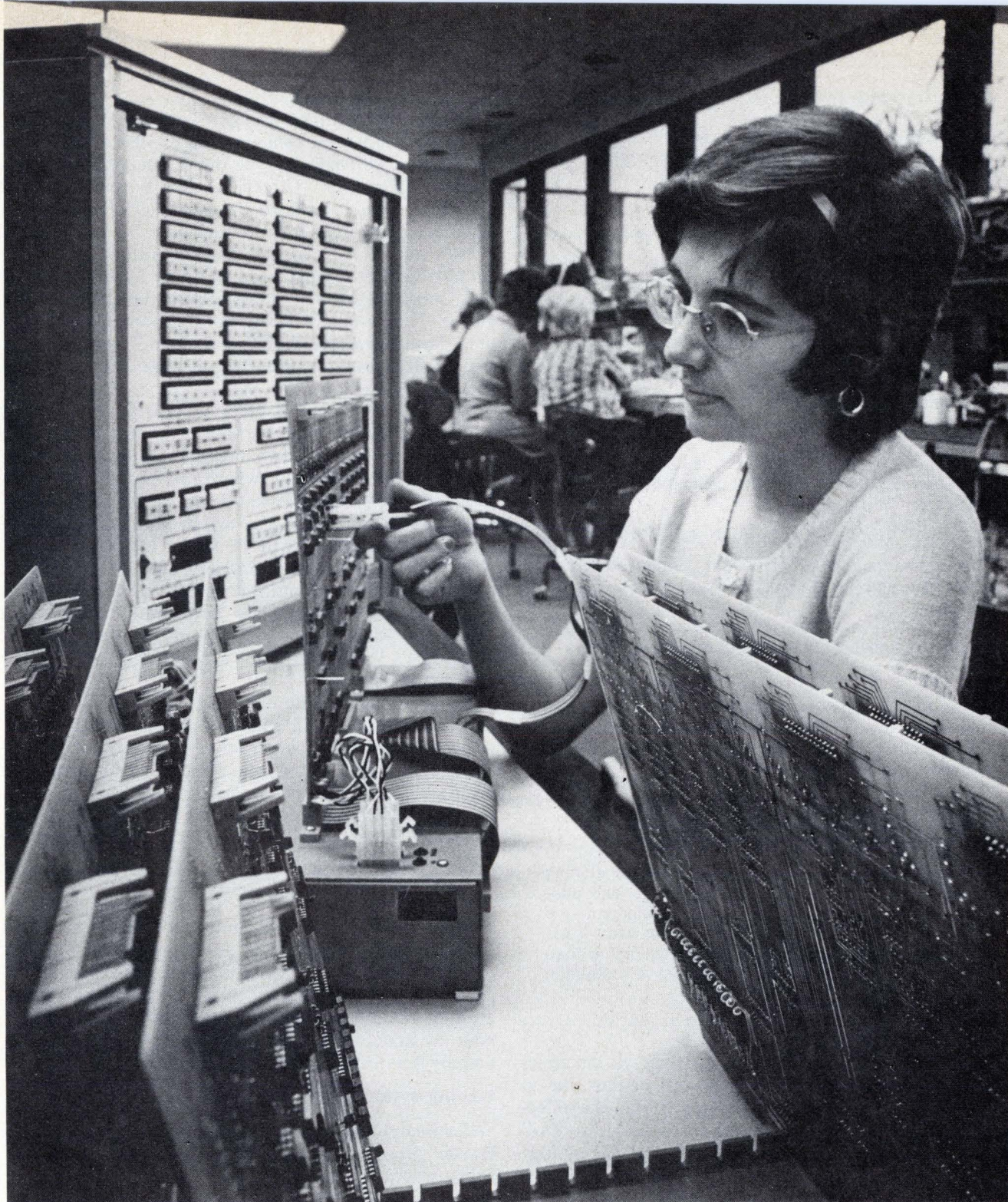
9. No software. The microprocessor of the Technology Marketing series 2000 tester is permanently programmed so that the user does not require any particular software. The operator enters the test procedure through switches and controls on the front panel. The procedure may then be stored on a magnetic card. Up to 700 test steps can be performed at a testing rate of 33 steps per second.
