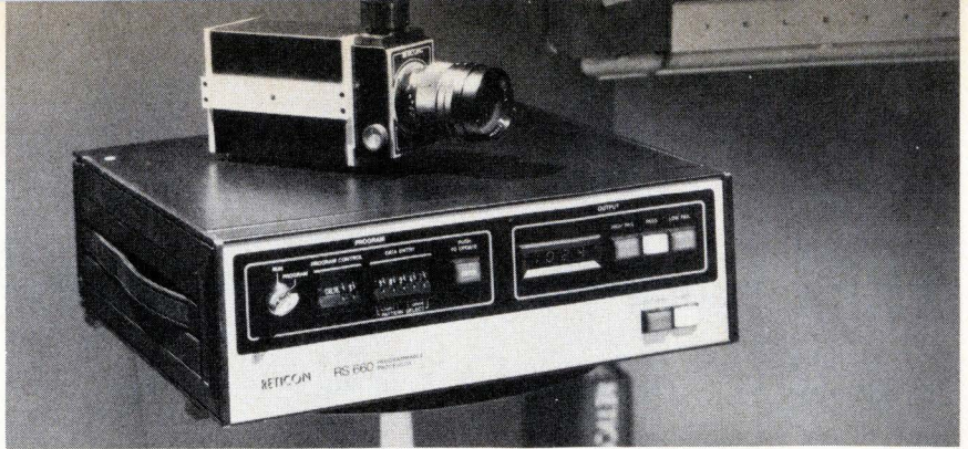
Smartie. Microprocessor-based controller helps solid-state camera make decisions.
