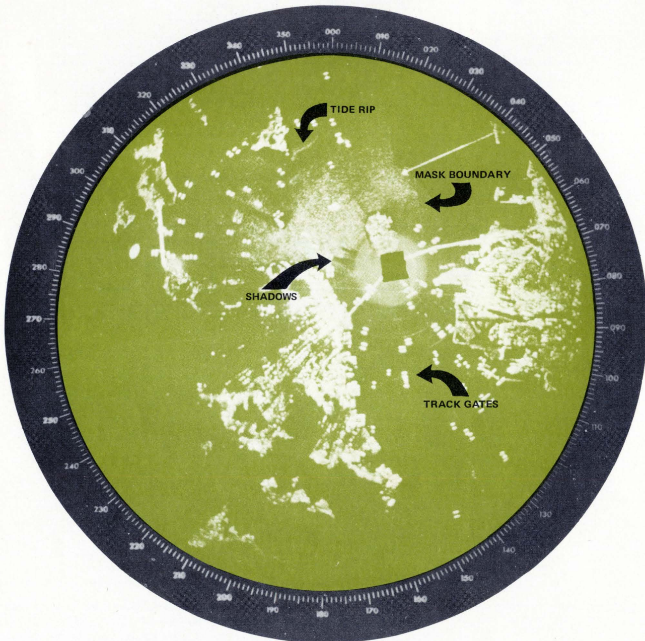
1. Bay area. The radar's plan-position indicator of the San Francisco Bay Vessel Traffic System shows ship tracks, as well as the undesired patterns caused by returns from irregularities in the tide-rip patterns. Parts of the area are deliberately masked out to reject returns from stationary objects.
