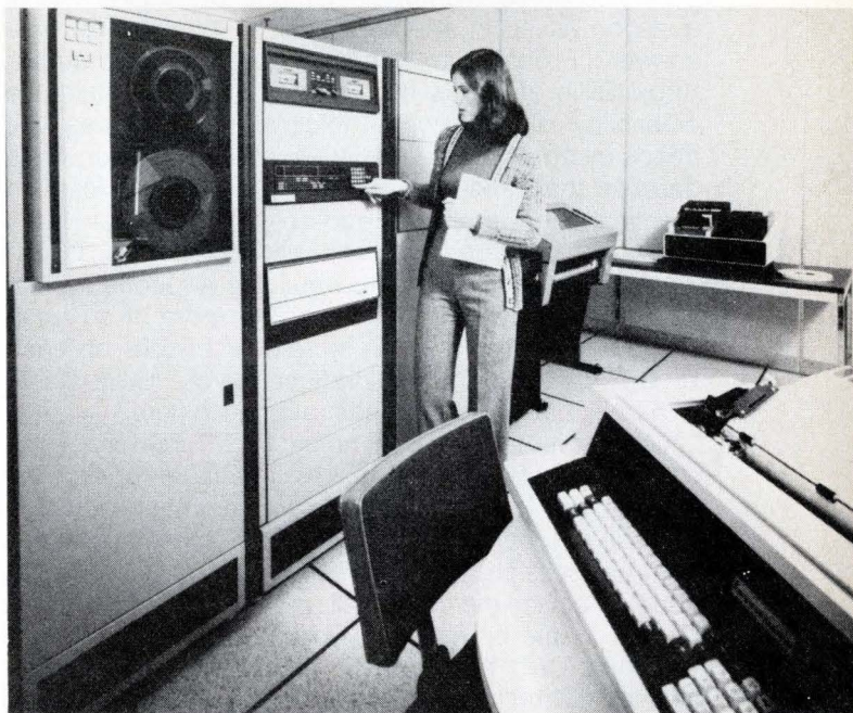
Trend-setter. New at NCC will be Interdata's 8/32 Megamini, a 32-bit machine with a 1-megabyte core memory in a single cabinet.
