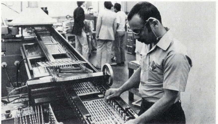
On their way. Top photo shows computer diodes being unrolled from shipping reels, while in bottom photo memory board is loaded onto belt of a wave-soldering machine.
