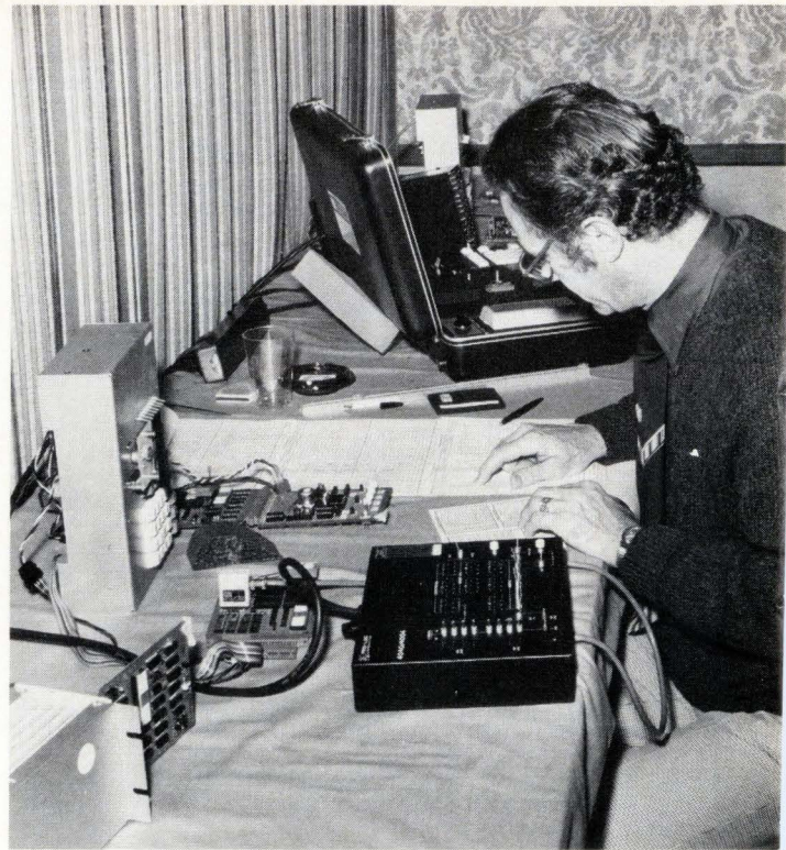
10. At the bench. Microprocessor systems—both hardware and software—can be checked out easily once the program has been fully documented, using the formats shown in Fig. 8 and a hardware system analyzer as shown here.
