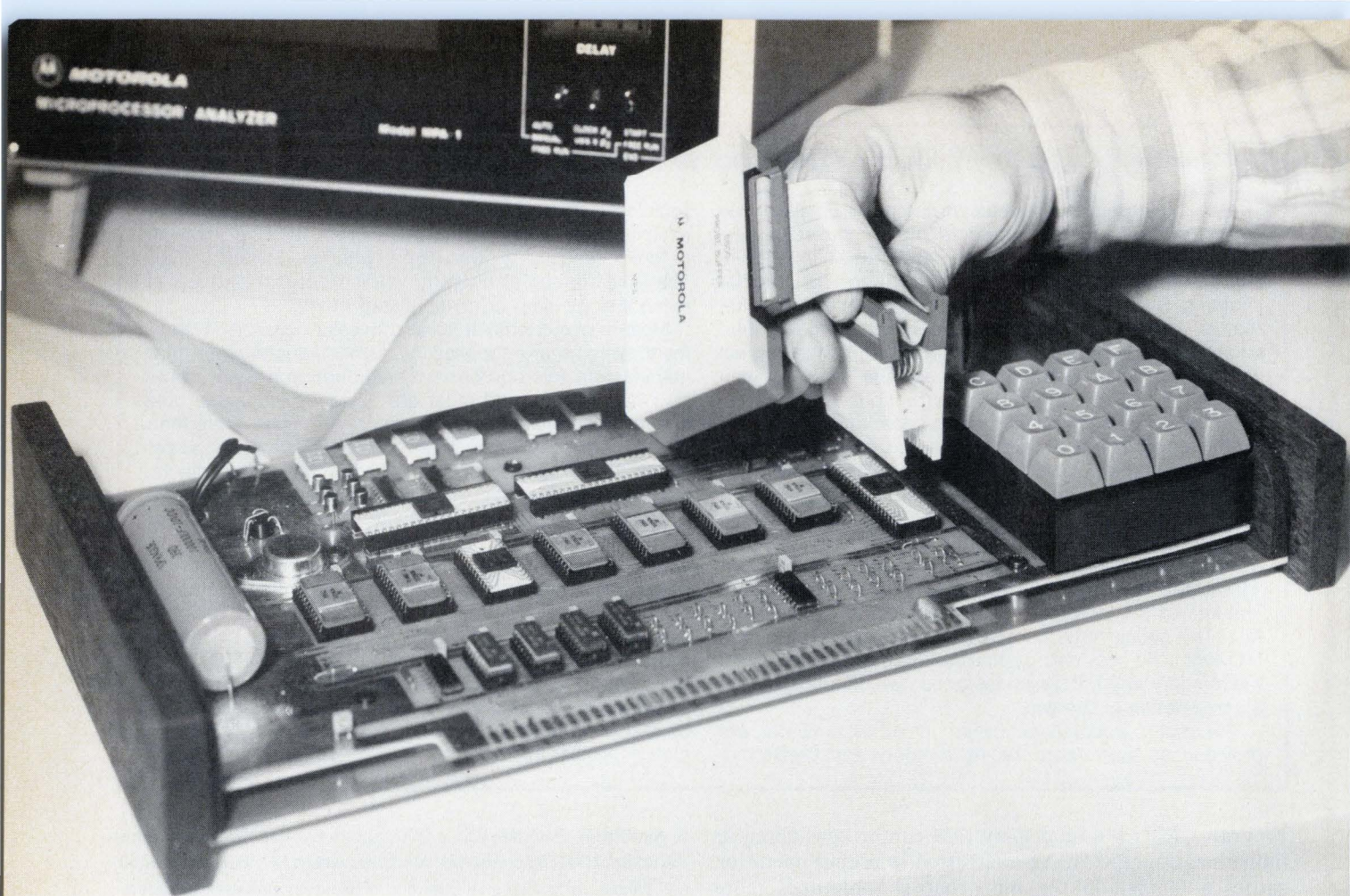
4. Clothespin. Microprocessor analyzers like Motorola's MPA-1 have conveniences like a single clip-on clothespin-like probe, which simplifies connecting the instrument to the circuit under test, and hexadecimal readout, which is easier to interpret than binary rotation.
