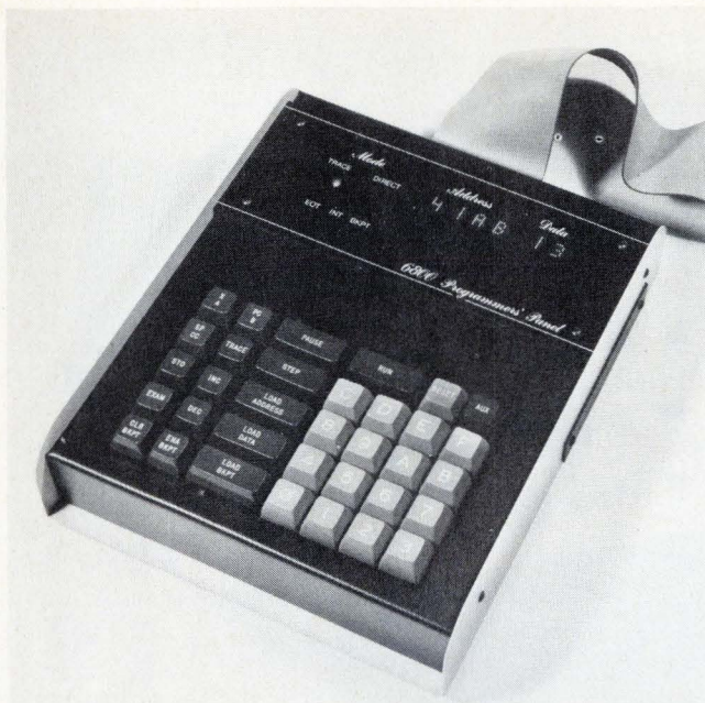
9. Interaction. By setting aside a portion of system memory and incorporating the appropriate connector, a designer can configure a microprocessor circuit so that the Applied Microsystems Programmers' Panel can retrieve or change internal registers.
