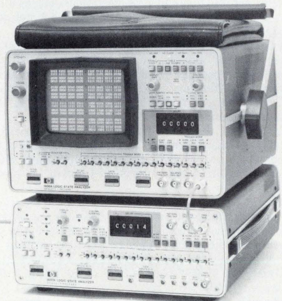
1. Doubling up. When used in tandem, the Hewlett-Packard 1600A and 1607A logic-state analyzers can display up to 32 channels of digital data in binary or map form to facilitate microprocessor-circuit testing. Up to 16 lines at a time appear on screen.
