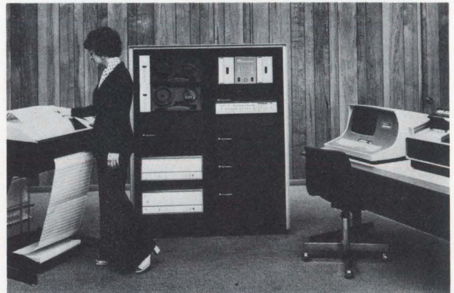
One million byte minicomputer by Computer Automation, pictured with high-speed disks, floppy disks, printer, card reader and CRT, comes with 224 instructions.
