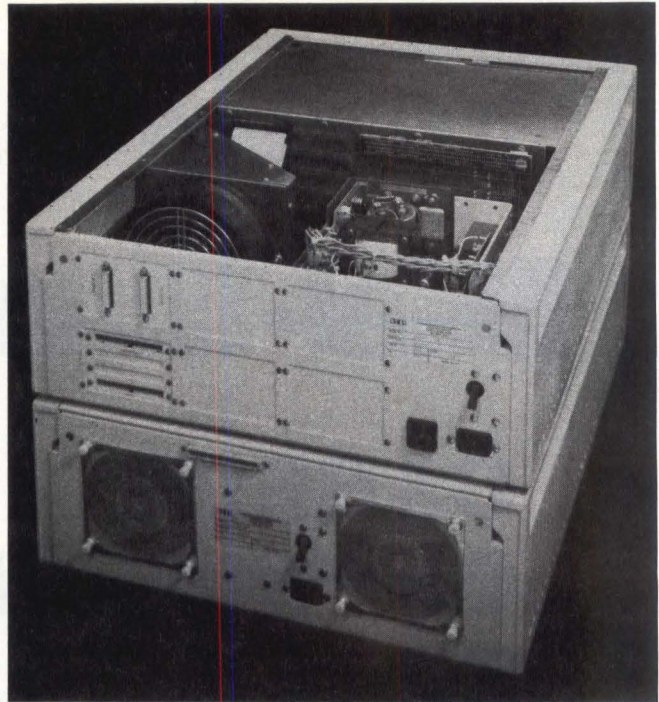
Charles River Data Systems' Universe (rear view, top removed) shows fan placement for horizontal cooling path. Vertical cooling, which is generally more efficient, is not practical for stacking components.
