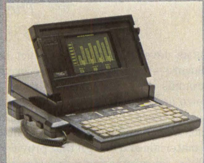
Grid System's Compass computer weighs about 9 lbs. and is smaller than a briefcase. Its magnesium case can withstand severe shocks.
