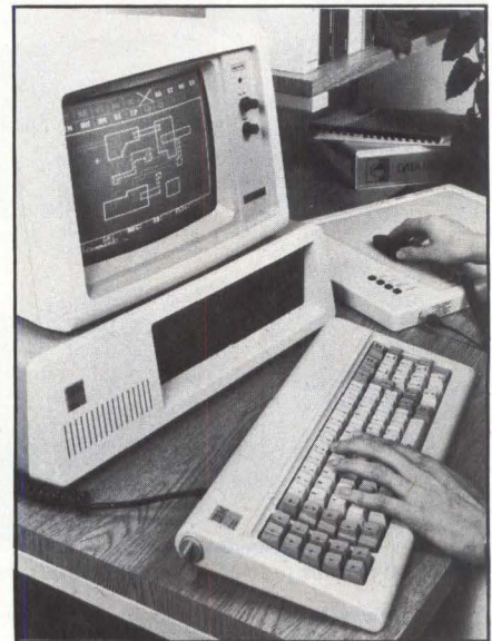
Color monitors for the Chancellor CAD workstation range in resolution from 320 × 200 to 1024 × 1024. The graphics software package is from CAD/CAM Technology, Sunnyvale, Calif.
