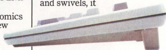
Low profile DIN-standard keyboard with adjustable tilt.
