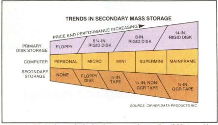
As a result of technology and price breaks, group-code-recording (GCR) tape drives can now be efficiently designed into computer systems smaller than mainframes.
