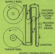
start/stop motion. As a result, vacuum-column drives increase tape speeds from 45 ips on tension-arm drives to 200 ips and beyond.
