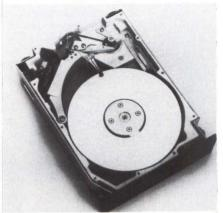
four-point shock mounting and internal diagnostics. All three drives use the ST-506/412 interface. Data-transfer rate is 5M bits per second; average access times are 95 msec. Model TL213: \$650 (500 units), model TL226: \$850 (500 units); model TL240: \$1,055 (500 units). Tulin Corp., 2393 Qume Dr., San Jose, Calif. 95131, (408) 942-9025.
