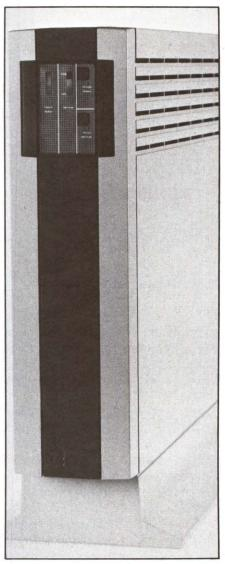
U.S. Design's 760M-byte VIP/X disk subsystem uses cache memory to speed access times and "bypass" slower electromechanical data-search processes.
