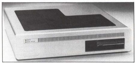
Seagate's 100M-byte ST-8100 Winchester disk drive (shown with the ST-9100 controller) is the company's bid in the high-capacity market. The ST-8100 takes the safe road in technology and manufacturability—an 8-inch form factor.
