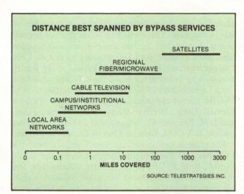
The efficiency of different types of bypass services varies with the distance spanned by a communication network. At one extreme, local area networks aren't able to span more than a few miles; at the other, satellite-based networks become efficient only when a network covers at least 700 miles, say most experts.
