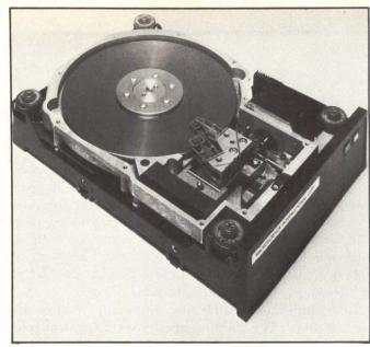
The HH-612 from Microscience International Corp. is one of the first half-height 5¼-inch Winchesters. The drive stores 10M bytes, has dual read/write heads on both sides of the disk and uses a closed-loop servo-positioning system. Price is \$580 in quantities of 2,500 to 5,000.
