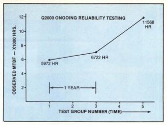
Fig. 8. The mean time between failures (MTBF) of the Q2000 drive consistently improved over time. The first test group rated the drive early in the production ramp. The 11,568-hour MTBF was recorded during full production.
