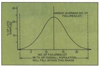
Fig. 1. Bell curve shows the failure ranges at the subassembly stage of drive assembly. Recorded failures in each lot sampled ranged from zero to 25, and the average number of failures was 12.5. The curve also measures the expected percentage of lots that fall into each number-of-failure category. Most lots had 10 to 15 failures. The area within the dotted lines determines the upper and lower control limits of each test level.
