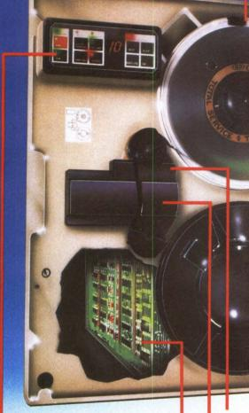
**EASY TO OPERATE:** touch sensitive switches and LED indicators with decimal readouts. Tape threading guides allow simple, fast loading.
