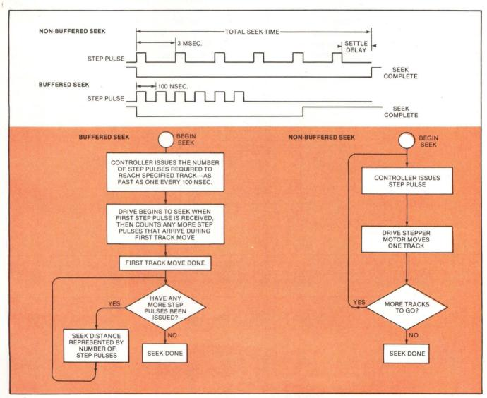
Fig. 4. Buffered seek can speed head positioning in stepper-based actuator systems. The microprocessor-based scheme allows a disk drive to accept all the step pulses for a seek at one time, thus keeping the stepping motor rotating. Non-buffered systems must accept one pulse, step the motor, stop and then accept another pulse before making another step. Buffered seek involves a more complex control procedure but significantly reduces access times.
