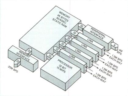
Inmos Ltd. has designed the Transputer 32-bit microprocessor chip to operate either standalone or in a network of Transputers. Each Transputer has four links that provide direct point-to-point communications with a link on any of four other Transputers.
