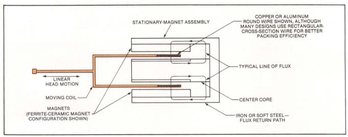
Fig. 5. A typical voice-coil motor works on principles derived from speaker technology. Just as in a standard acoustic speaker, current in the moving coil produces a magnetic field, which pushes against a permanent field in the stationary magnet assembly. Because the moving force is proportional to the amount of current in the coil, a smooth, easily controlled linear movement is produced.
