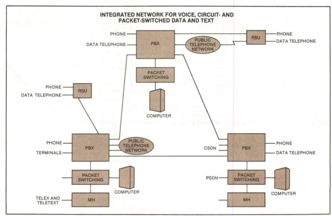
In this network that integrates voice and data, several remote PBX systems are linked over leased digital telephone lines. Such a network might connect a company's buildings within one city, for example. RSU stands for an extension of the main PBX, called a remote-switching unit, PSDN is (public) packet-switched data network, CSDN is circuit-switched data network, and MH is a message handler for telex or teletext. (Source: Ericsson Information Systems A.B.)
