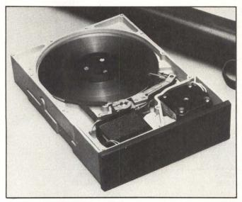
Tandon's half-height TM250 Winchesters offer 6.4M or 12.8M bytes of unformatted storage. The drives use plated media and a rotary stepper motor. The plating consists of a nickel and cobalt layer on an aluminum substrate.
