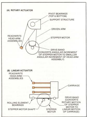
Fig. 3. Stepper-motor-driven actuators, like their high-end voice-coil relatives, come in rotary (A) and linear (B) configurations. Both types of rotary and linear systems employ approximately the same mechanisms. Voice-coil designs, however, use servo loops and feedback information to achieve precise head positioning.
