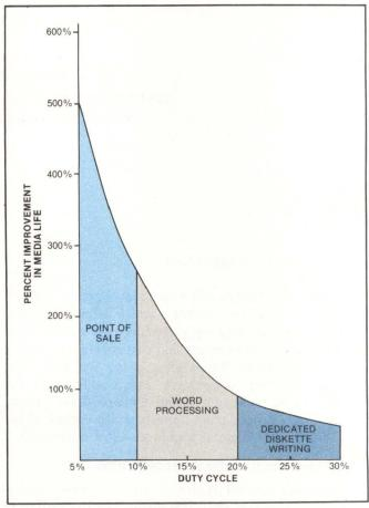
Media-life improvement using a fast-start motor rather than a head-load mechanism depends on the disk drive duty cycle (percent of system time that a drive is reading or writing). The lower the duty cycle, the greater the improvement in media life, but all applications benefit from some improvement. The data shown are based on the assumption that heads contact six tracks at a time when loaded and that contact with the most-frequently-accessed track occurs 50 percent of the time.
