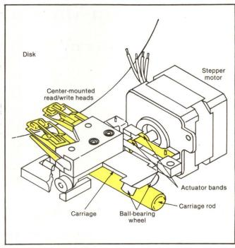
Fig. 3. The head/carriage assembly includes center-mounted read/write heads that move in a straight line toward the center of the disk. The carriage moves along one carriage rod as opposed to two rods, as in most drives.
