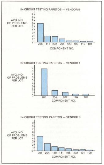
Fig. 3. Pareto charts graph recorded failures by type and frequency. Codes on the x-axis are Quantum Corp.'s internal codes identifying each failure mode. (Each of the charts applies to a different vendor.)
