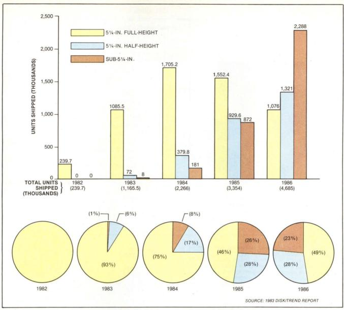
Fig. 2. Full-height drives dominate the less-than-30M-byte, 5¼- and sub-5¼-inch Winchester market. Half-height drives will reach production quantities this year and are expected to gain 17 percent of the market. Provided that standards are established for sub-5¼-inch drives by 1985, they are expected to dominate the market by 1986 with a 43 percent share, representing more than 2 million units shipped. Figures are for the worldwide market and include captive and OEM markets.
