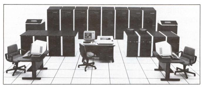
Tandem Computers Inc. says its 32-bit NonStop TXP system performs at least twice as fast as other Tandem systems. A system with two CPUs, 4M bytes of main memory, two 128M-byte disk drives and software sells for \$328,550.
