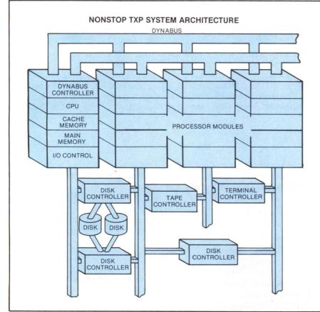
Tandem's NonStop TXP system comprises two to 16 processors, a proprietary Dynabus, dual-ported controllers and multiple shared power supplies.
