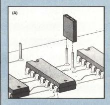
The physical implementation of jumper options affects the ease of reconfiguring a disk drive. Three kinds of implementations are common: a shorting plug, a shunt pack and a cut/jump trace.
