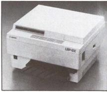
The Canon LBP-CX laser beam printer puts all printing functions, except for a semiconductor laser imaging system, in a removable cartridge. Canon is selling the device with a video interface to OEM customers.
