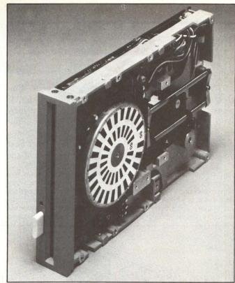
Canon U.S.A.'s MDD221 diskette drive measures 1.32 inches high, 5.9 inches wide and 8.7 inches deep. The double-sided, double-density drive holds 1M byte.
