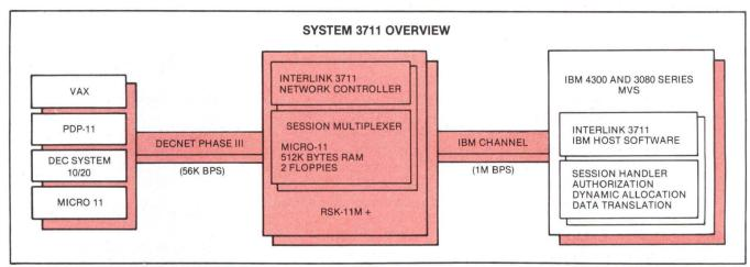
The Interlink System 3711 connects a DECnet with IBM/MVS systems without the use of JCL. Prices start at \$98,500.
