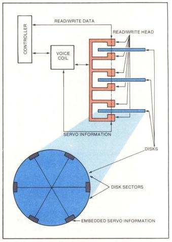
Fig. 7. An embedded closed-loop servo system codes servo information at the beginning of each Winchester disk's data sector, freeing all of the disks for data.
