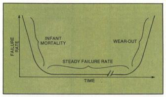
Fig. 2. A bathtub curve shows failure rates of a product over time. In the beginning, "infant mortality" results in a high failure rate. After burn-in, the product exhibits a steady failure rate during its operating life. Finally, the product begins to wear out, and the failure rate increases sharply.
