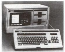
connection to the host or a printer. The model 1625 is host-compatible with the HP 3000. It has an application-specific keyboard and provides an HP terminal personality with block-mode capabilities. The model 1631 has a DEC VT100 terminal personality and complies with the ANSI X3.64 standard. \$3,995 each. Delivery is 60 days after receipt of order. Direct Inc., 4201 Burton Dr., Santa Clara, Calif. 95051, (408) Circle No 302 980-1414.
