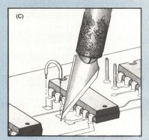
mounted on an IC socket can easily be removed and replaced.
