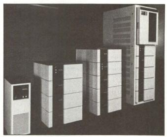
Supermicrocomputers that run the ICS Ada compiler include models 11, 21 and 31 of Zilog's System 8000. One of the model 31s shown includes an optional nine-track tape drive.
