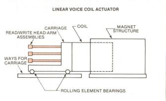
least six sets of ball bearings (four to guide the mechanism and two for anti-rotation), compared with the two bearings that rotary devices use.
