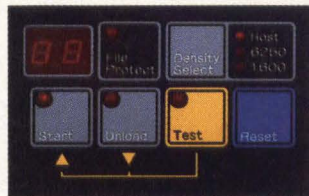
Operator panel displays fault codes for easy troubleshooting.
