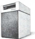
For PDP-11/04-60 UNIBUS: 300 MB Removable Emulates DEC RM05
