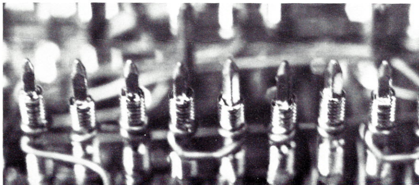
Examples of good wire wrapping.
