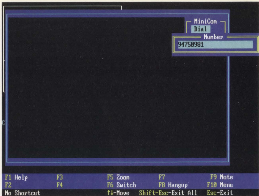
Figure 3. MiniCom accepts a phone number from the user through a prompt defined in the .PRO file.
